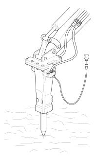
Position the hydraulic breaker vertically towards solid bedrock or similar to adjust the pressure using a pressure gauge.
