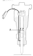
Lubricate the working tool's shank plentifully during all upward operations. The bushing and the working tool must be lubricated so frequently that dirt cannot penetrate into the hydraulic breaker.
