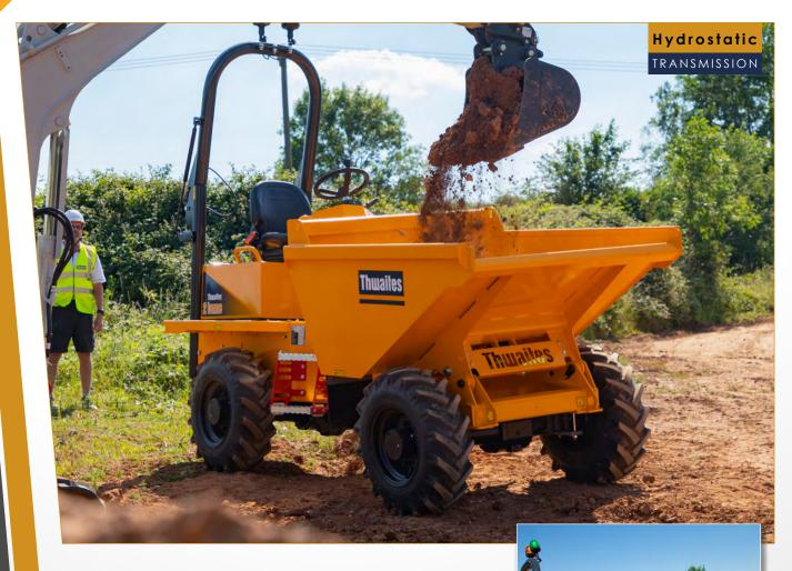
The Thwaites 2 Tonne Front Tip, Stage V dumper is manufactured with contractors and hirers in mind - ensuring operator safety, reducing risk on site and improving performance. Powered by an 18.1 kW 3-cylinder Yanmar engine, delivering 107 Nm max torque for optimum traction and control. The Thwaites 2 Tonne Front Tip is also available with a Manual
