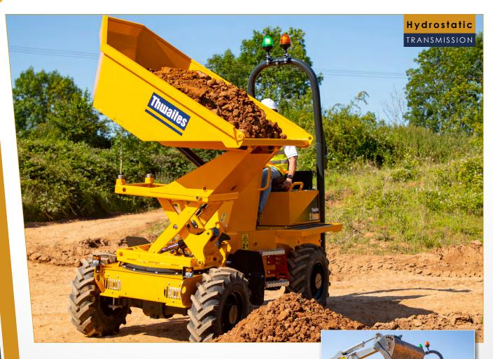
The Thwaites 2 Tonne Hi Swivel, Stage V dumper is manufactured with contractors and hirers in mind – ensuring operator safety, reducing risk on site and improving performance. Powered by an 18.1 kW 3-cylinder Yanmar engine, delivering 107 Nm max torque for optimum traction and control, this machine is driven by a Hydrostatic transmission, making it simple and straightforward to operate.
