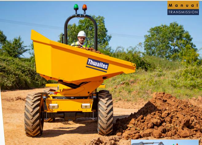
The Thwaites 3 Tonne Power Swivel, Stage V dumper is manufactured with contractors and hirers in mind - ensuring operator safety, reducing risk on site and improving performance. Powered by an 18.1 kW 3-cylinder Yanmar engine, delivering 107 Nm max torque for optimum traction and control. This machine is driven by a Manual transmission.
