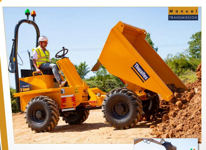
The Thwaites 3 Tonne Front Tip, Stage V dumper is manufactured with contractors and hirers in mind – ensuring operator safety, reducing risk on site and improving performance. Powered by an 18.1 kW Yanmar engine, delivering 107 Nm max torque for optimum traction and control. This machine is driven by a Manual transmission.
