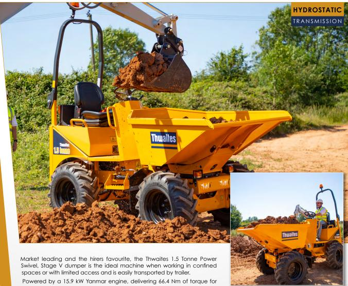
Powered by a 15.9 kW Yanmar engine, delivering 66.4 Nm of torque for optimum traction, this dumper is driven by a Hydrostatic Transmission making it very easy to operate.
