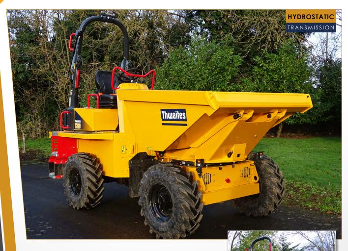
The Thwaites T350 Power Swivel, Stage V dumper is manufactured with contractors and hirers in mind – ensuring operator safety, reducing risk on site and improving performance. Powered by a 33.3 kW Yanmar engine, delivering 142 Nm max torque for optimum traction and control, this machine is driven by a Hydrostatic transmission, making it simple and straightforward to operate.
