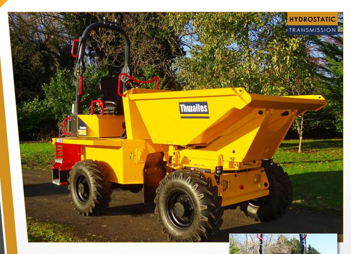
The Thwaites T300H Hi Swivel, Stage V dumper is manufactured with contractors and hirers in mind – ensuring operator safety, reducing risk on site and improving performance. Powered by a 33.3 kW Yanmar engine, delivering 142 Nm max torque for optimum traction and control, this machine is driven by a Hydrostatic transmission, making it simple and straightforward to operate.
