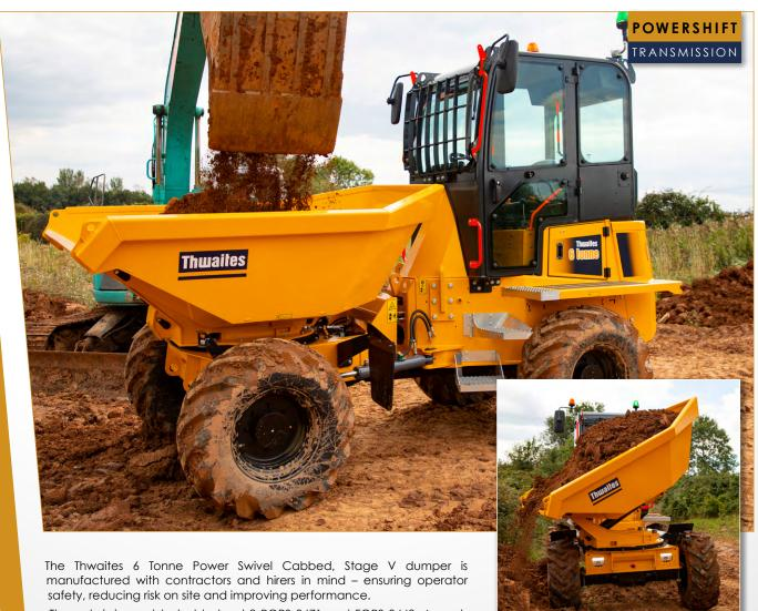
The cab is impact tested to level 2 ROPS 3471 and FOPS 3449. As such all Thwaites cabbed dumpers are approved for use by the UK Major Contractors Group. The Power Swivel skip enables a 90° rotation left and right, allowing the machine easier access to tip loads in restricted areas, giving the operator greater control and reducing risk on site.
