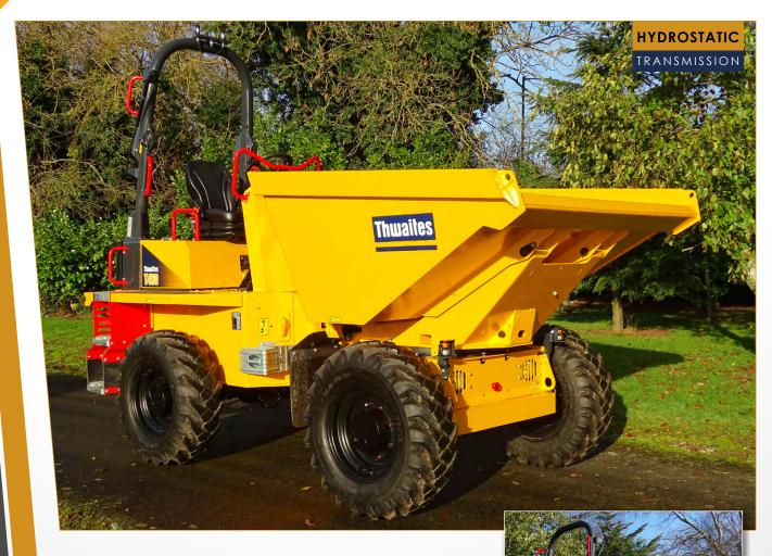
The Thwaites T450 Power Swivel, Stage V dumper is manufactured with contractors and hirers in mind – ensuring operator safety, reducing risk on site and improving performance. Powered by a 33.3 kW Yanmar engine, delivering 142 Nm max torque for optimum traction and control, this machine is driven by a Hydrostatic transmission, making it simple and straightforward to operate.
