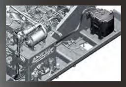
Added electric heating wire to urea piping An electric heating wire has been added to the urea piping to prevent urea from freezing in cold regions or in winter.
