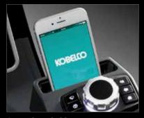
Smartphone holder You can use the holder with your smartphone connected to the USB port.
