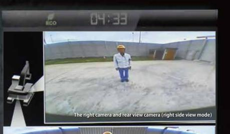
The right camera and rear view camera (right side view mode)
