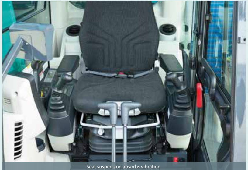
Seat suspension absorbs vibration
