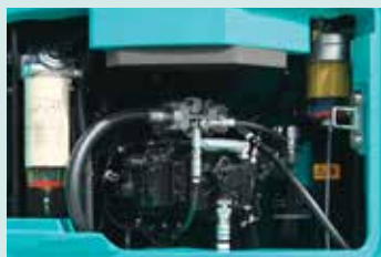
Fuel filter with built-in water-separator
