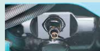
Engine oil quick-drain valve can be turned without special tool.
