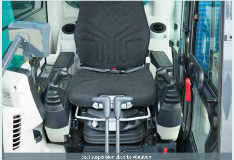
Seat suspension absorbs vibration
