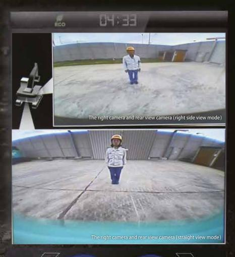
The right camera and rear view camera (right side view mode)
